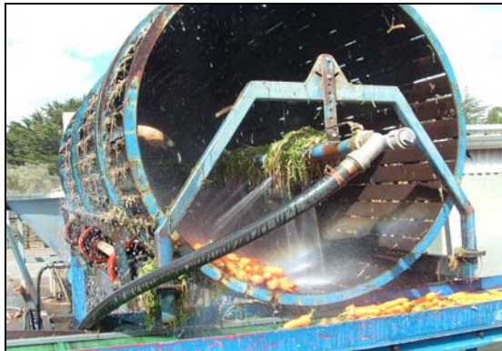
Figure 5: Farm #2 – Carrot tops are removed in a large tumbler outdoors, while being sprayed with stream water.
