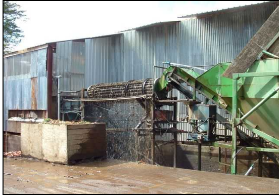
Figure 4: Farm #1 - Carrots arrive in big green hopper and are rinsed with stream water in a tumbler outdoors.
